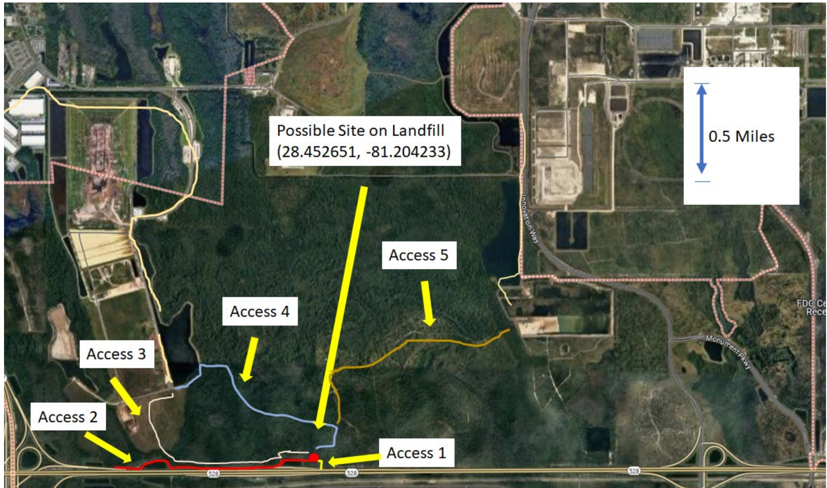
Illustration of potential access routes to the Orange County landfill site (Visual Aid Identifier 1), including existing maintenance roads and potential gated easements from the 528 Toll Road.
